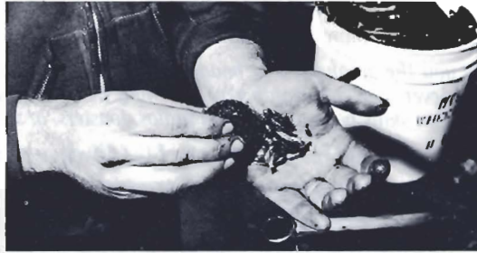
8. Repack wheel bearings as shown. This factory-recommended procedure is messy, but effective. Replace wheel bearings if they appear worn or "corrugated."
