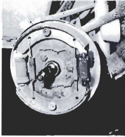
7. Once the new shoes are in place, be sure all the parts you removed are back on the assembly. Worn return springs should be replaced.
