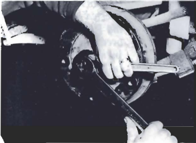
9. Now replace the drums on the assemblies. It is essential that the axle nut be very tight; the factory recommends 200 pounds of torque. Proper tools help get the job done easier.
