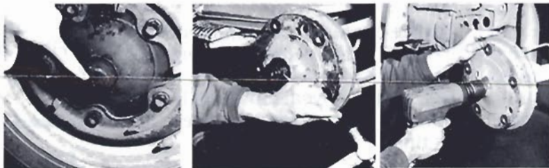
1. Begin the brake project by removing all wheels. Speedometer cable tab must be removed from the left front wheel before the drum can be removed.
