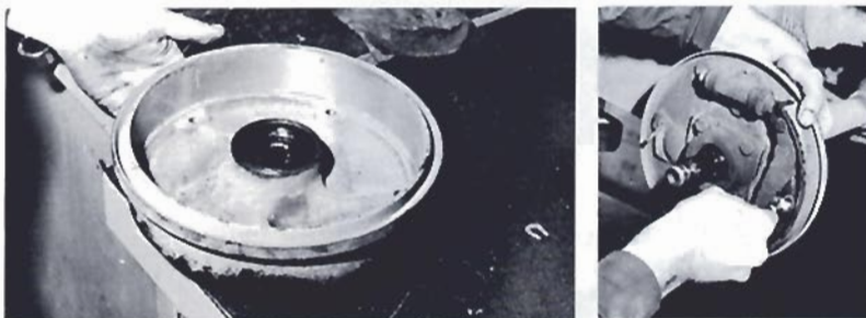
5. Brake drums should always be sent out to be "turned" before installing new brake shoes. This will assure proper mating of the shoes to the drum surface.
