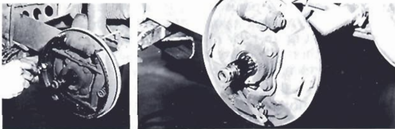
3. Inspect the shoes to see if they must be replaced. If they are worn, remove them by depressing the small retainer clips with a screwdriver or pliers.
