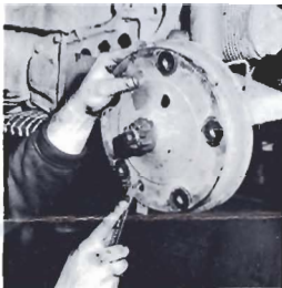
11. Adjustment holes for late-model VWs with 4-bolt patterns are located on the back side of the brake drum assembly. Earlier models are adjusted on the front side.
