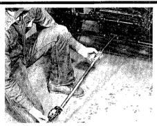
Using a crow bar, bend the cable housing tubes as far out of the way as is possible. On late model chassis you may have to remove the internally welded seat belt securing nuts from the inside of the tunnel to make enough room for the linkage retaining frame.
